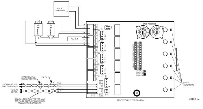
\*NOTE 1: To audio amplifier supervision EOL device. Refer to Control Panel Installation Manual for wiring instructions
