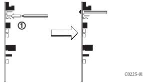
Step 1: Install two long standoffs in the lower mounting holes using two 4-40 nuts as shown.
