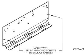
The BB-XP cabinet has a built-in chassis that will accommodate one or two XP6-C modules.
