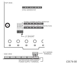
NOTE: SLC wiring is the top terminal block, notification appliance/power supply is the bottom.
