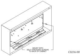
The BB-XP cabinet comes with the chassis already installed, so no mounting is necessary.
